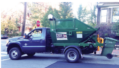
Cambridge, MA uses rear-loading, semi-automated trucks for its curbside collection program.
